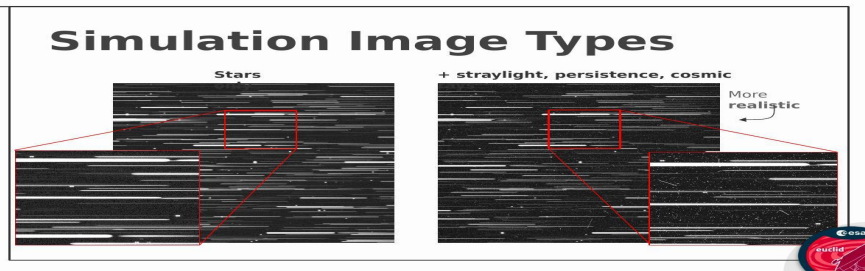
Euclid SPV: stars only (left) vs full noise model including stray light, persistence and cosmic rays (right).
